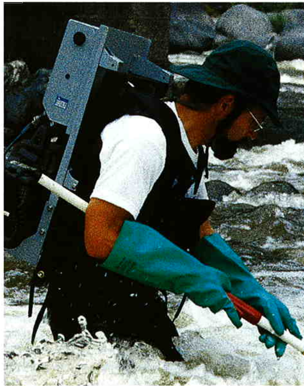
The Academy's ichthyology collections manager, Dave Catania, uses an electroshocker to stun fishes in the Bajiao River in Yunnan, China.
