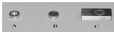
FIGURE 1: Mini-mesocosms in aluminium stubs of 4 mm height and 10 mm diameter. The cavities are 3 mm in depth and 6 mm in diameter (A). Small aliquots of thoroughly homogenized sediment samples are transferred into the cavities of aluminium stubs (B). These can be placed in humid chambers under defined conditions of e.g. light, temperature and salinity. After cryofixation, the stubs are mounted onto a specimen holder (C) and transferred into cryochamber attached to a scanning electron microscope.
